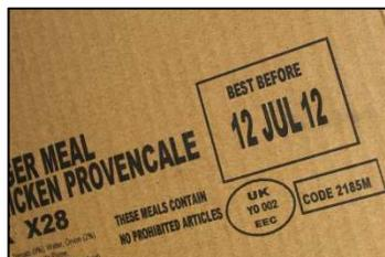
One of the many solutions used in today's production facilities to meet the needs of identifying cases of various products is the use of labels, both pre-printed and printed on-demand.
